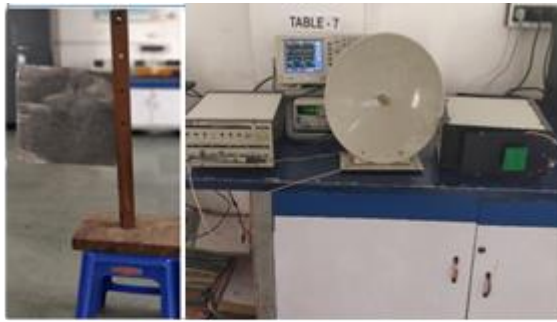
Fig 2-Prototype of Measurement setup for SAR/ISAR System
